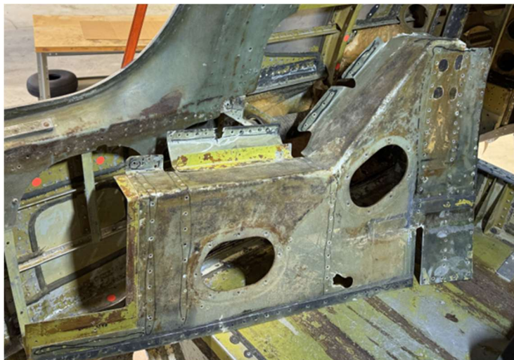
Right Duct – Loose Ready for Removal
