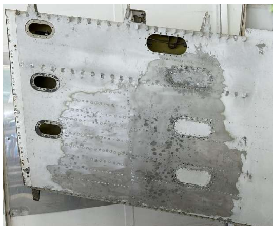
Corrosion Area on Left Lower Wing Skin
