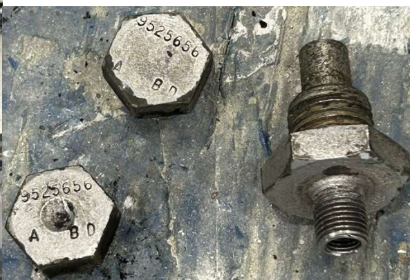
Left: Two Fuse Plugs. Right: Inflation Fitting
