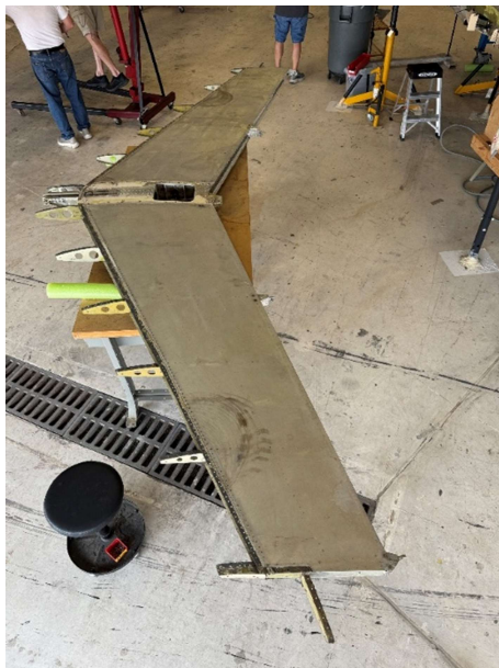
Horizontal stabilizer with Leading Edges Removed
