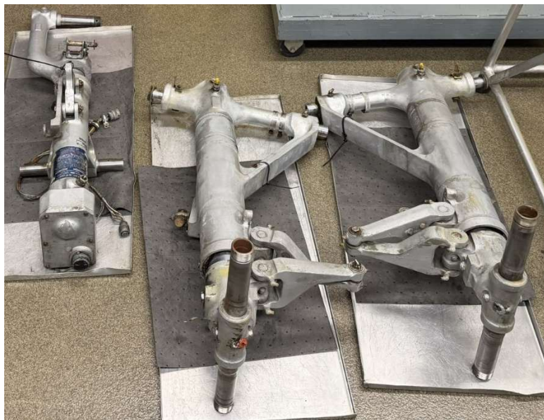
Landing Gear, Cleaned and Ready for Disassembly
