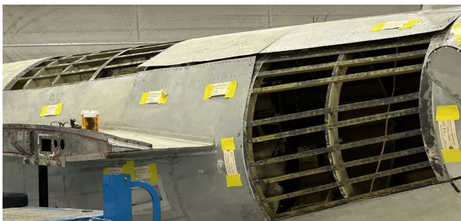
Two Aft Fuselage Skins Now Removed
