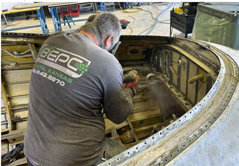
Ryan Timesch working on forward pressure bulkhead
