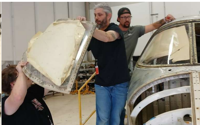
Left Windshield Removed Trenton Lindsey, Trevor Peacock, Terry Brodek, Jr
