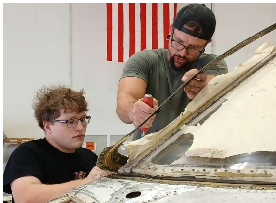
Removing Windshield Retainer Trenton Lindsey, Terry Brodek, Jr
