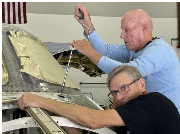
Jim Tidball, Al Goodwin (blue shirt) removing windshield screws
