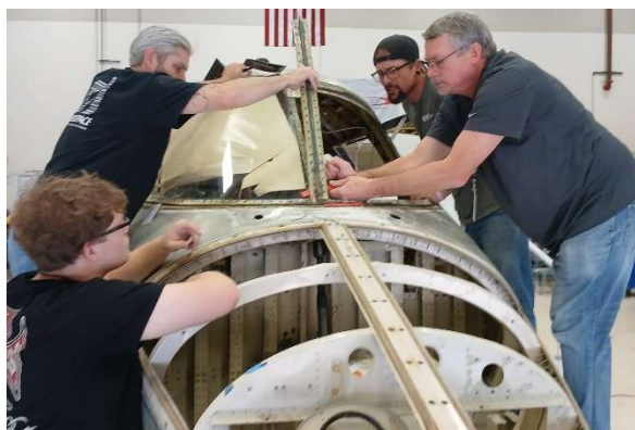
Removing the Center Post Trenton Lindsey, Trevor Peacock, Terry Brodek, Jr, Tim Walker
