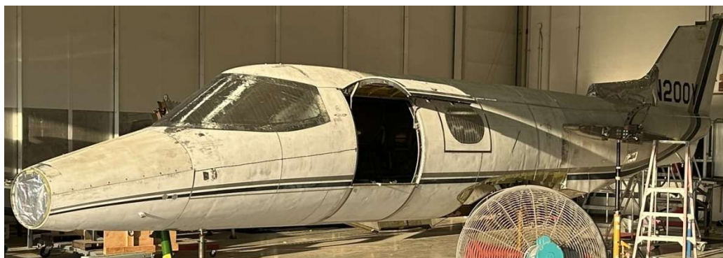
Fuselage Left Side - aluminum tape on windshield, seams and dorsal fin
