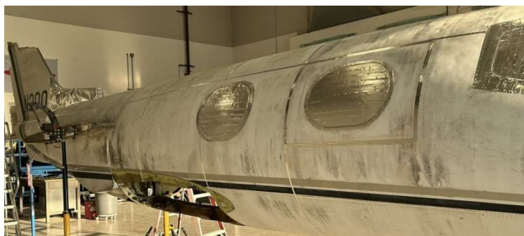
Fuselage Right Side - aluminum tape covering windows and seams
