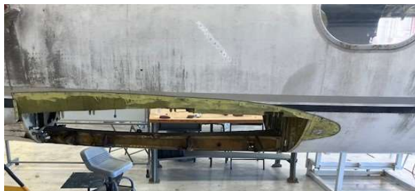
Keel Beam and Emergency Exit Door Reinstalled
