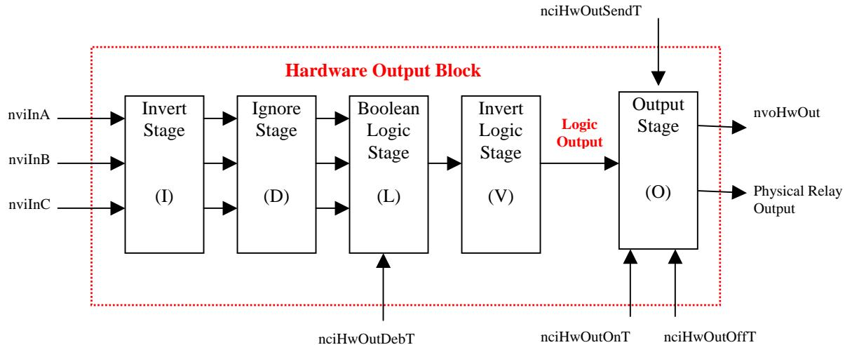
The Model 2150 firmware contains four Hardware Output Blocks. The output of each block controls the corresponding physical relay output. The Blocks are highly configurable but simple to use. Hardware Output Blocks have the following features:
