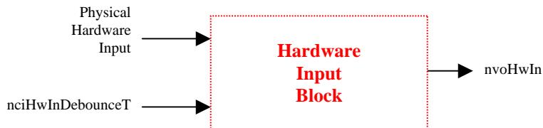
The Model 2150 contains four Hardware Input Blocks. A diagram is shown above. The block receives its input from the physical hardware. A configurable debounce time can be set via the nciHwInDebounceT network variable. The output of the block is available using nvoHwIn Output Network Variable.
