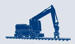
The S Series Rail Guidance System has retractable rail wheel assemblies that are installed on the excavator, positioning the vehicle on the rail while allowing the tires to continue to provide traction and braking. The blade has a mechanical twist mechanism to meet Australian Standard.
