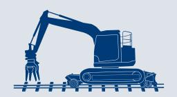
The S Series **Hi Rail System** can be set to either narrow, standard or broad gauges. A single manually operated valve is installed to switch from track to rail mode while still allowing the excavator to operate in travel mode.
