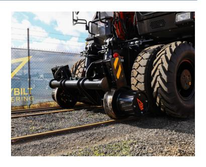
Released in 2019, the Hi Brid was designed locally by Harrybilt Engineering's specialist team of railway maintenance equipment engineers. Since 2001, the company has been designing and manufacturing Hi Rail and Rail Guidance Systems for road rail vehicles. In addition to this, the team have years of experience in manufacturing equipment for the rail industry since 1985.
