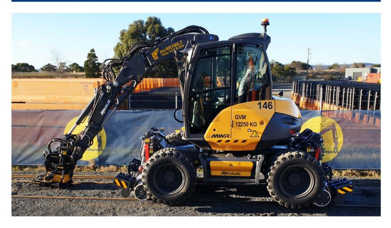
Harrybilt Engineering have developed a customised rail system. The Hi Brid allows a wheeled excavator to run on both standard and narrow gauges.
