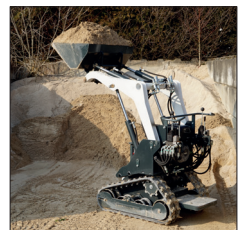
2015, microBull lifting height 130 cm
