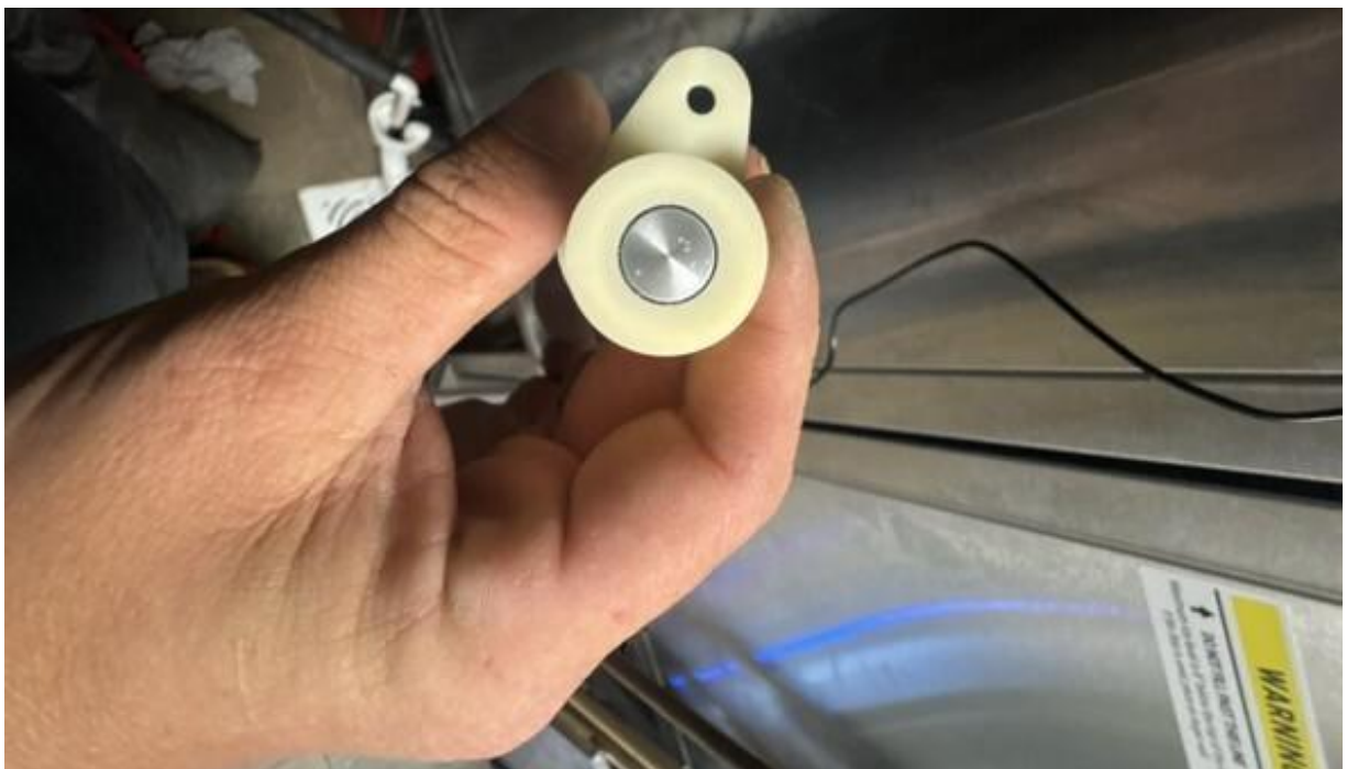
Cleaning a Hoshizaki UltraSonic bin sensor
