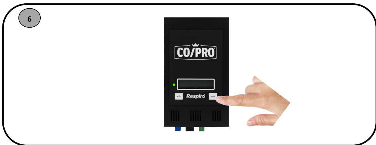
**Step 6**—The CO/PRO will take approximately 1 minute to go through its warm-up process. Once the device is ready, press the “Mute” button for greater than 6 seconds to activate the test mode. Verify that the alarm is working, the red light is flashing, and that all connected devices (furnace and water heater) were powered off by the CO/PRO. When the CO/PRO’s operation has been validated, press the “Mute” button for greater than 6 seconds to put the CO/PRO into its ready state.
