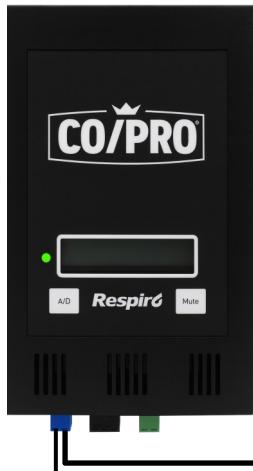
When using the CO/PRO to only monitor the supply air from a furnace, the “blue” connector on the CO/PRO can be connected to a an alarm panel that accepts a normally closed (NC) contact. In this configuration, the CO/PRO will “open” the contact when 25 ppm of CO is detected, thereby providing an alert to CO in the ambient air. When the CO level decreases to 15 ppm or less, the alarm will be cleared and the CO/PRO’s contact will return to a normally closed state (NC)
