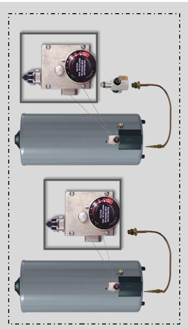
**Step 4**—Use an existing or new 120/24 VAC transformer to bring 24V (AC) to power the CO/PRO. Manual pilot water heaters require a thermocouple junction block (not included) be inserted between the thermocouple and the water heater's control box (see picture above) to connect to the CO/PRO. For automatic pilot water heaters, splice into the Flame Sensor High Temp wire and connect each end to the CO/PRO.
