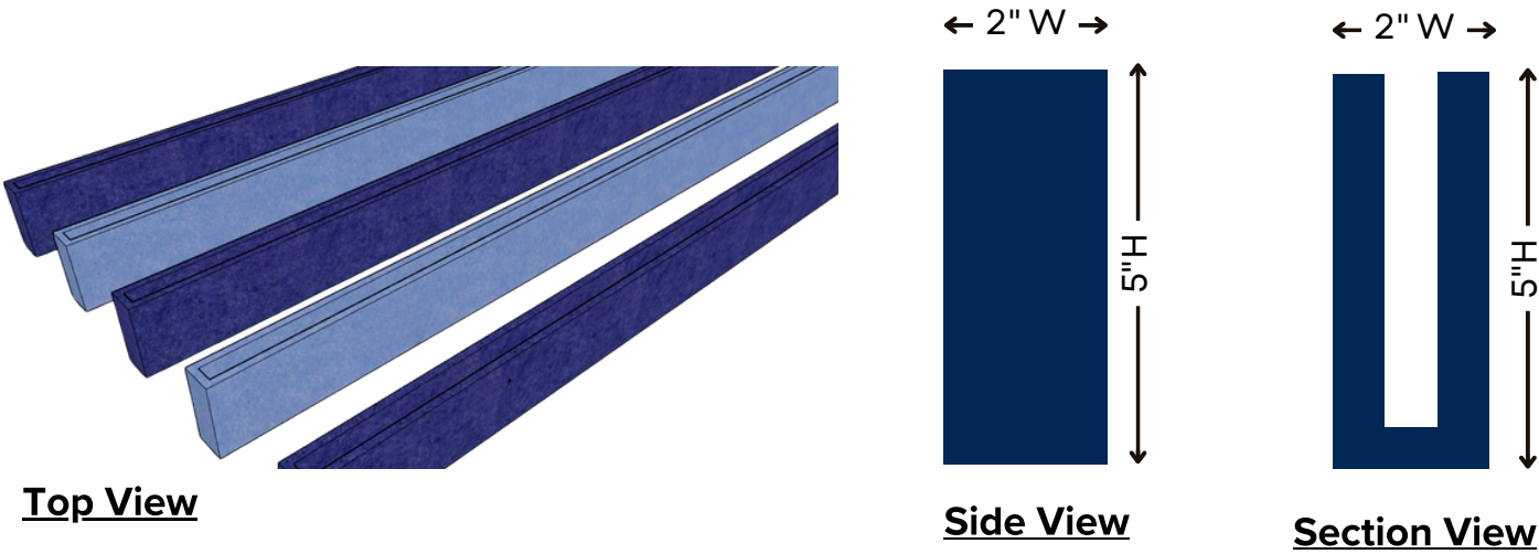
Perspective View of the Fuselage Box Beam Baffles
