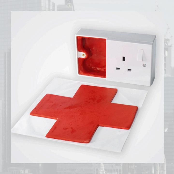
Putty pads are flexible, fire-resistant sheets that are designed to safeguard electrical socket boxes installed into plasterboard walls. They are made from silicone-based polymers, and they are applied inside or around the electrical socket boxes to restore the fire rating of the wall. When exposed to high temperatures, the pad expands to for a protection, sealing off gaps and preventing fire and smoke from spreading.
