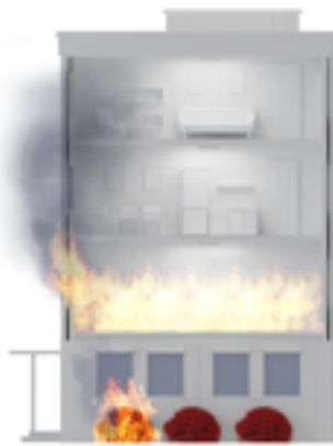
60 minutes: Fire contained within cavity compartment 1
