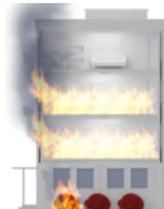
90 minutes: Fire contained within cavity compartments 1 and 2
