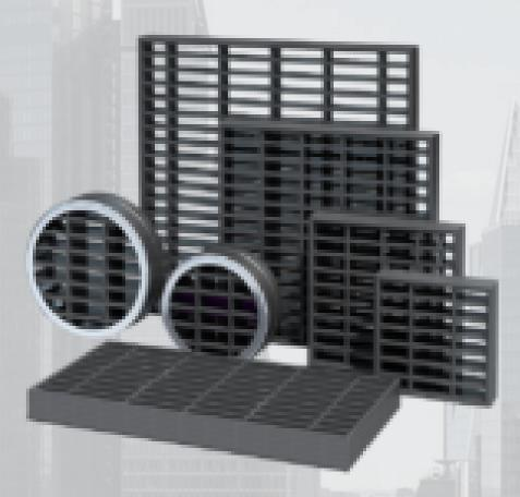
Designed for fire-rated doors, walls, and ducts, this product allows free airflow under normal conditions. In a fire, the intumescent material expands to seal openings, forming a solid barrier.
