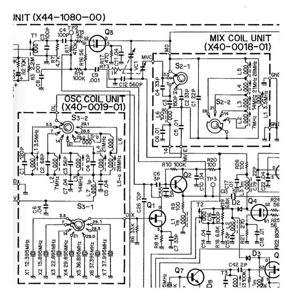
I prefer to know what I am trying to do and why. That frees me to do things differently if I need to. Knowing how the circuit works makes odd things stick out in a design. For instance, notice the odd section of wafer switch S3-1. Why does the switch have that split double wiper contact for the crystal selection?
