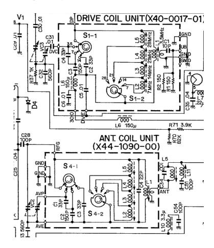
This is not the way all the coils are, though. On the same board, there is S2-2 with shunted coils, but S3-2 are not shunted. These coils can be tweaked independently of each other. So you have to look at the schematic to understand what you are trying to do.
