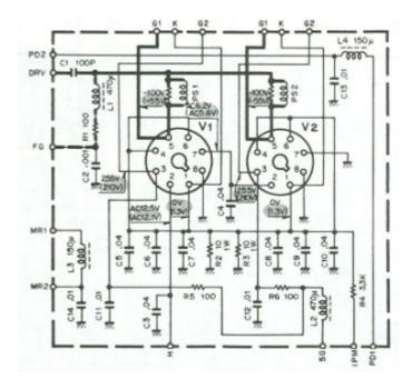
Here's a nice picture by Ken, K4EAA. It shows a final cage diagram of the TS-820. It is pretty much the same as the TS-520, down to the 100 pF driver coupling capacitor. I use this picture because Ken does a beautiful job.
