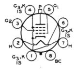
Whenever I hear about 6146's oscillating, that's the first thing I check for. Something is not grounded that should be. The 6146 is a high gain tube, meaning if it doesn't know where ground is, it will take off and never come home. It will spread it's glorious 6146 wings, and take along with it, any resonant thing or things nearby, and make that it's new oscillatory home.
