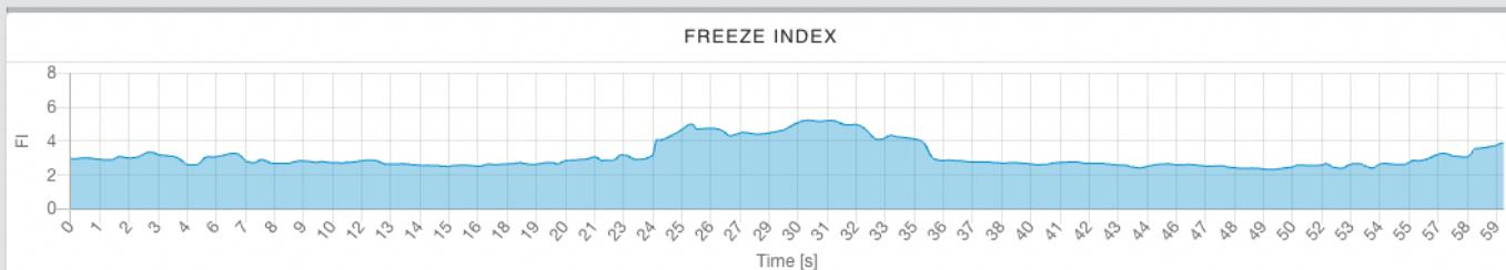
The freeze index (FI) shows the likelihood of freezing at a given moment in time. If the user freezes, the FI shows a higher value, as shown in the figure between 24-36s.
