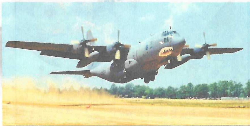
A C-130 Hercules goes airborne. It's a four-engine turboprop military transport aircraft produced in many variants.
