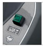
Reverse mow switch enables you to carry on cutting in reverse at the same speed so you can be as efficient as possible, it then resets itself when you move off forward again.
