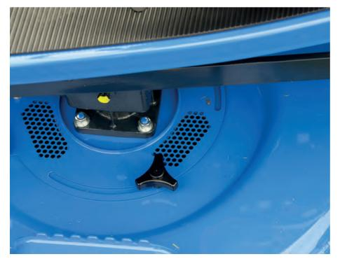
Using the vents on the top of the decks you can open or shut these to control the airflow from the deck to the collector to allow as much cut grass and debris as possible to be drawn through, this is especially useful in winter when you have a lot of wet heavy grass. In the summer you can close it up to minimise the dust and debris being kicked up when mowing in very dry areas.
