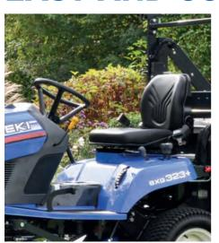
Simple to drive, the 2-pedal hydrostatic control allows for the ultimate control so you can quickly change direction and speed whilst mowing with minimal effort. The large operators platform offers maximum comfort with plenty of leg room, ergonomic controls and suspension seat.
