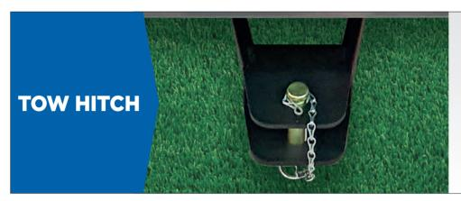
Tow hitch is available to enable you to move a trailer around behind the SXG mower, available whether you have a collector fitted or not.
