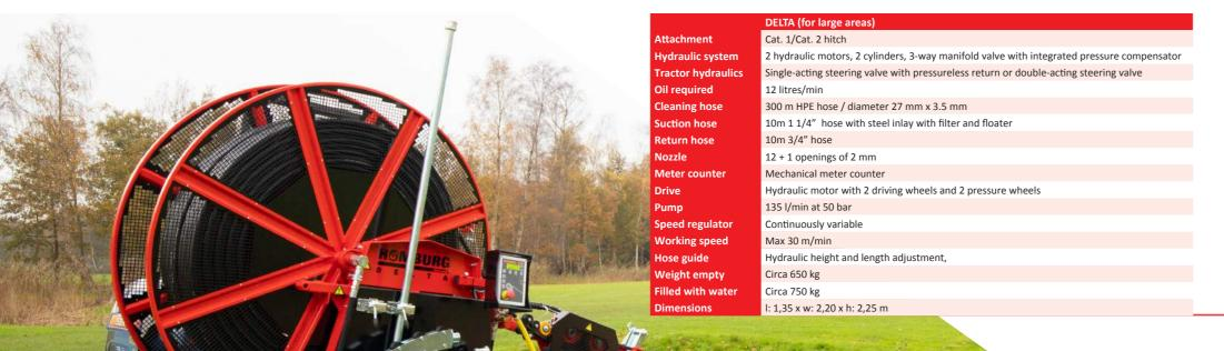
The Delta offers more ease of use as a draincleaner than the Blizz. This is the ideal machine for anyone who maintains drainage systems on a frequent basis and needs to cover a larger grounds. This is because it offers hydraulically operated height adjustment, extension, retraction and folding of the drainage arm and length adjustment of the guide arm.
