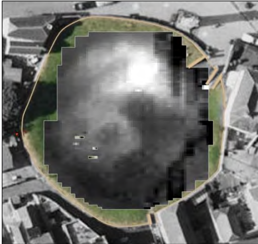
FIGURE 17: RESULTS OF AN EARTH RESISTANCE SURVEY AT ST JUST 32 .
