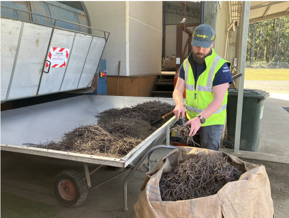
Figure 10 Removal of a rotating-drum kiln charge at the DEECA seed extraction facility at Orbost [Photo: Caitlin Cruikshank, DEECA]
