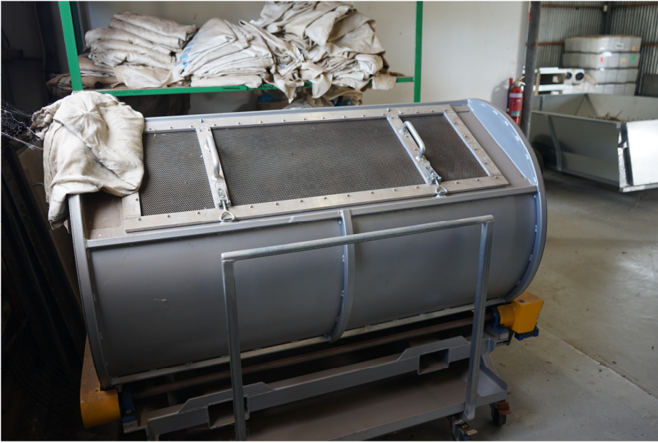
Figure 9 Seed extraction container at STT designed for extraction of smaller capsule collections. This modular unit can be used together with the main kiln. A much larger rotating drum unit is used for larger capsule crops.
