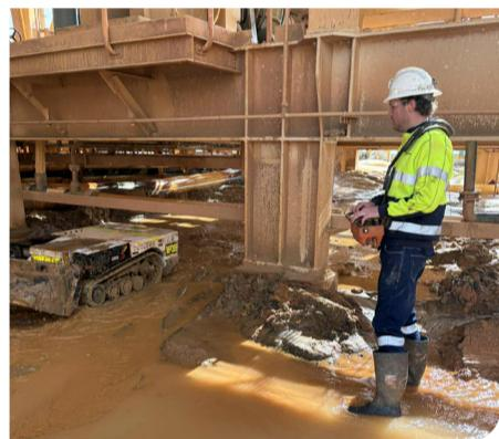
By reducing the need for personnel to enter hazardous areas, MPC minimises exposure to confined spaces, dropped objects, dust and material flow hazards while achieving faster and more consistent cleanup results.
