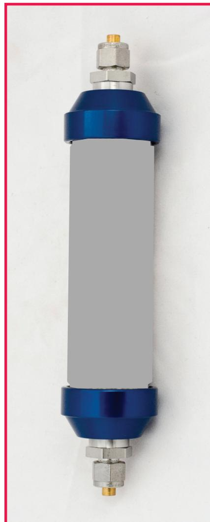
Gas traps should be mounted in a vertical position to ensure proper contact of the gas with the adsorbent. Use model 6400C or 8040C mounting clip with 6400 Series carbon dioxide trap.
