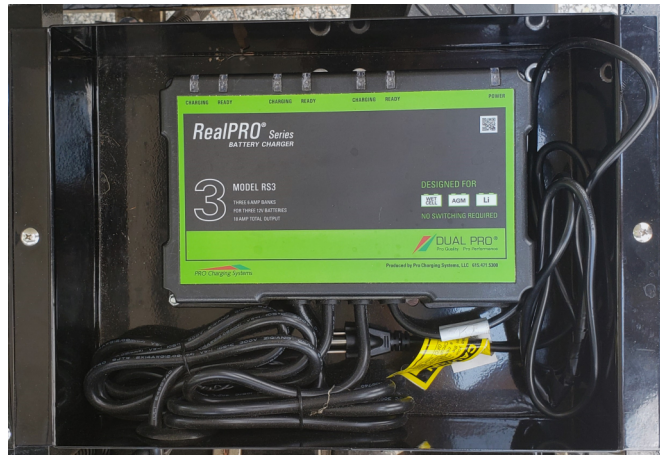
Three Bank Charger
