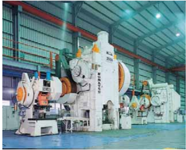
Forging Press 2500 tonnes & 1000 tonnes capacity
