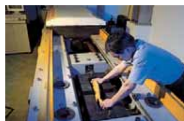
Tensile Test, Capacity 300 tonnes
