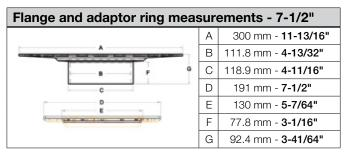
The 6" (150 mm) round/square grates are not compatible with the flange with 5-1/2" (140 mm) adaptor ring.
