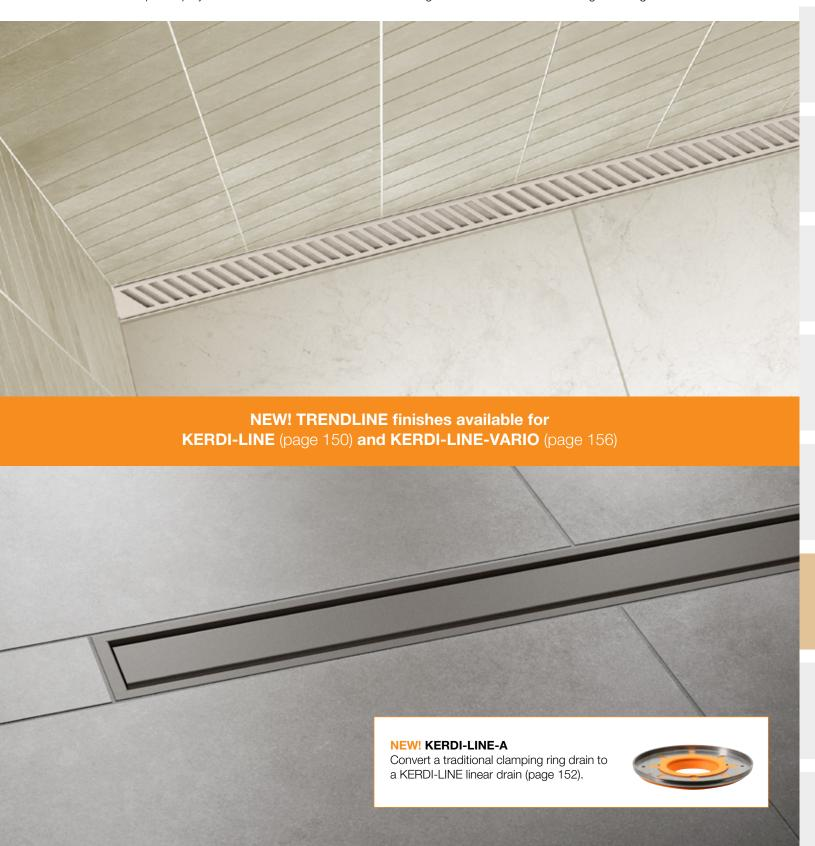
The Schluter®-KERDI-LINE is a low profile linear floor drain specifically designed for bonded waterproofing assemblies. KERDI-LINE can be installed adjacent to walls or at intermediate locations in showers, wet rooms, and other applications that require waterproofing and drainage. The floor can be sloped on a single plane to KERDI-LINE, which enables the use of large-format tiles and creates interesting design opportunities.
