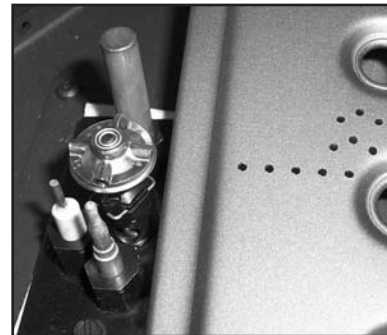
Figure 15: Burner to pilot hood relationship.
