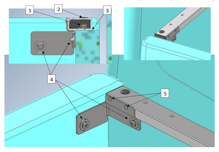
6 - Fit a M6 x 50 s/s bolt, flat and spring washer to the centre 'locking hole'. Fit one of the Nylon packers to the rear of the side rail on the M6 x 50 bolt.
