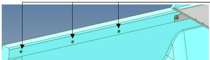
5. Remove the remaining 3 bolts from each side of the tub.
