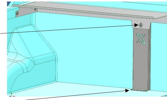
Once fastened, drill 2 @ Ø5 holes at the bottom of the support and pull up 2 @ 5mm S/S rivets.
