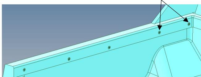
2. Carefully slide the infill into place. Fasten the sides with 2 @ M6 x 25 S/S button head socket screws, penny & spring washers (each side) into the factory holes.
