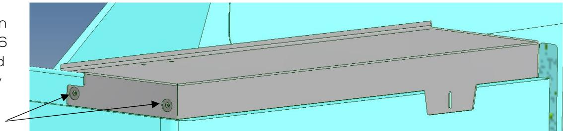
3. Fit the centre infill brace using 1 @ M6 x 25 S/S button head socket screw, spring & penny washer (top of brace has a M6 rivnut fitted).
