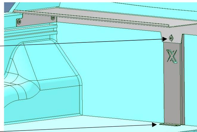
4. Seal the infill to the tub all the way around using Silicon. Smooth off and remove any excess (This MUST be done well to avoid any water ingress).
