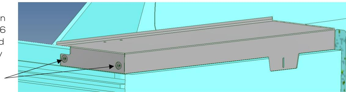
3. Fit the centre infill brace using 1 @ M6 x 25 S/S button head socket screw, spring & penny washer (top of brace has a M6 rivnut fitted).
