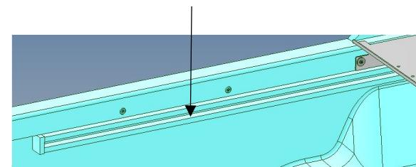
6. Remove the remaining 3 bolts from each side of the tub.
