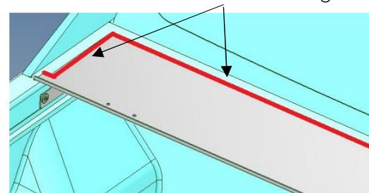
5. Remove the side tie rails (these will interfere with the S/S side rails).
