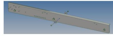
9. Remove the 2nd plastic clip back from the cab on the side of the tub. Insert an M6 x 25 socket screw / M6 penny washer (through side rail / tub liner) M6 penny washer / M6 nylock nut in each side rail after fitting to lock in place.
