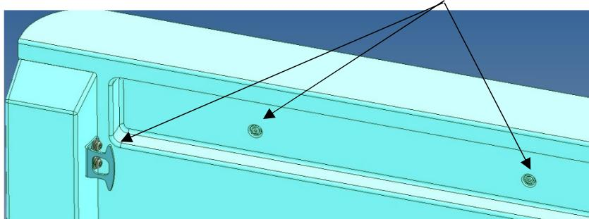
10. Fit side rails using 2 @ M6 x 40 S/S button head socket screws / spring & penny washers. Refit rear tie hooks using 2 @ M8 x 40 S/S button head socket screws / spring & flat washers.
