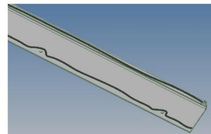
7. Sit the 2mm ali infill panel in place. Align the Ø5 holes to the main infill panel using the Ø5 S/S rivets supplied, pull up all 5 rivets.
