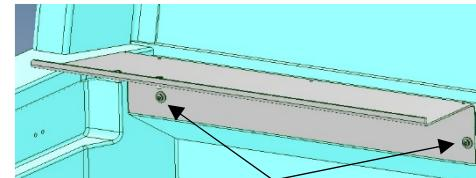
2. Fit infill using 3 @ M6 x 40 S/S button head socket screws / spring & penny washers.
