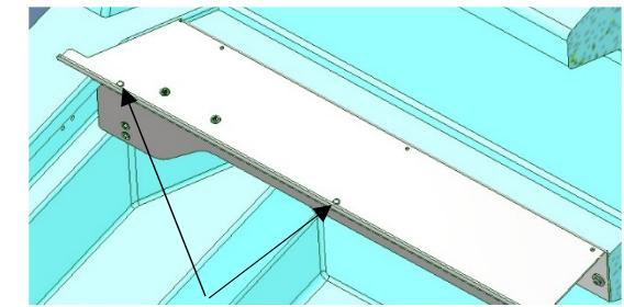
4. Rivet infill stiffener in place using 4 @ Ø5 S/S rivets.
