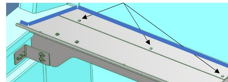
9. Remove the rear tie hooks and 2 side bolts.
