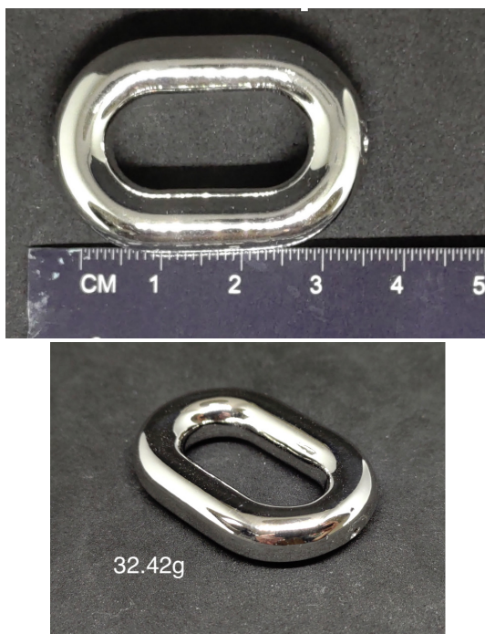
Figure 9: Platinum Electroformed piece of 1000 microns (1mm) thick, weighing at 32.42g
