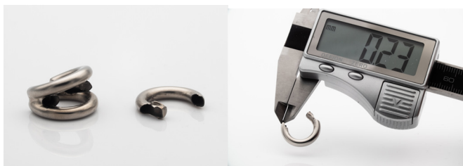
Figure 13: Ear accessory that snapped under pressure, wall thickness at 230 micrometers.
