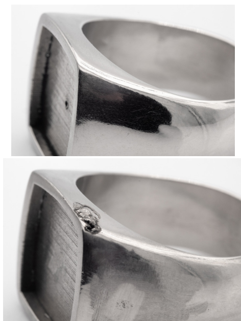
Figure 7: Deterioration in electroforming surfaces include porosity, pits and pox like bubbles. Most often shows up on flat surfaces where deposition occurs at a slower rate compared to corners. Ring electroformed from the 1st run of a bath (top), compared to a ring formed from the 3rd run of the same bath. (bottom)
