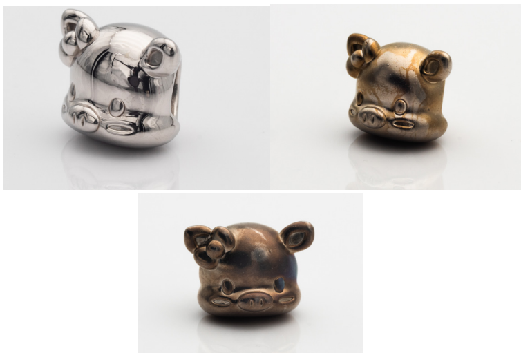
Figure 8: System B electroformed products, charm from 1st run polished (top left), the 10th run unpolished (top right), the 15th run unpolished (bottom).
