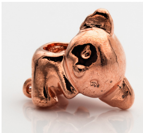
Figure 3: mandrel casted in low melting alloy
