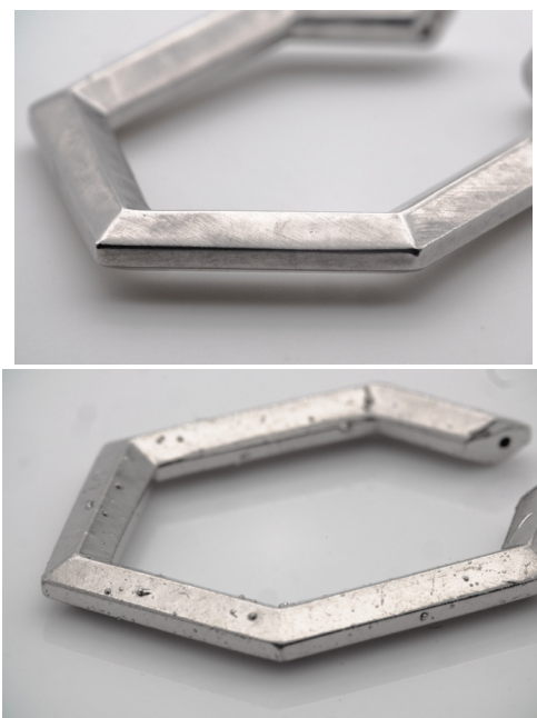
Figure 6: comparison of platinum surfaces after 1 run (on the left) and 3 runs (on the right).
