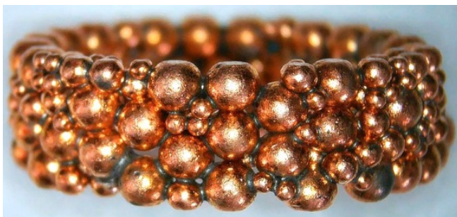
Figure 23. Ring made by liquid phase sintered mixed spheres deformed approximately 20% with a platen press.
