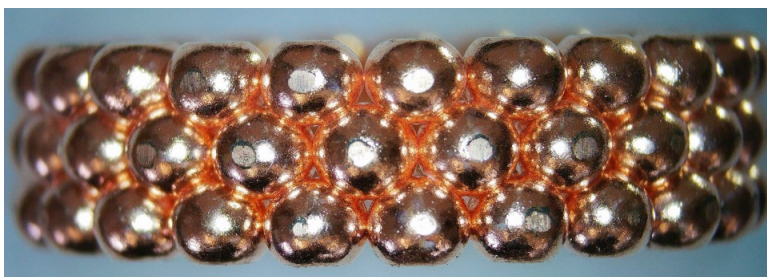
Figure 14: Ring made from 3 mm spheres compacted approximately 30%.
