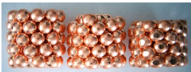
Figure 13: Cylinders of 3 mm spheres deformed 10%, 20%, and 30% left to right.
