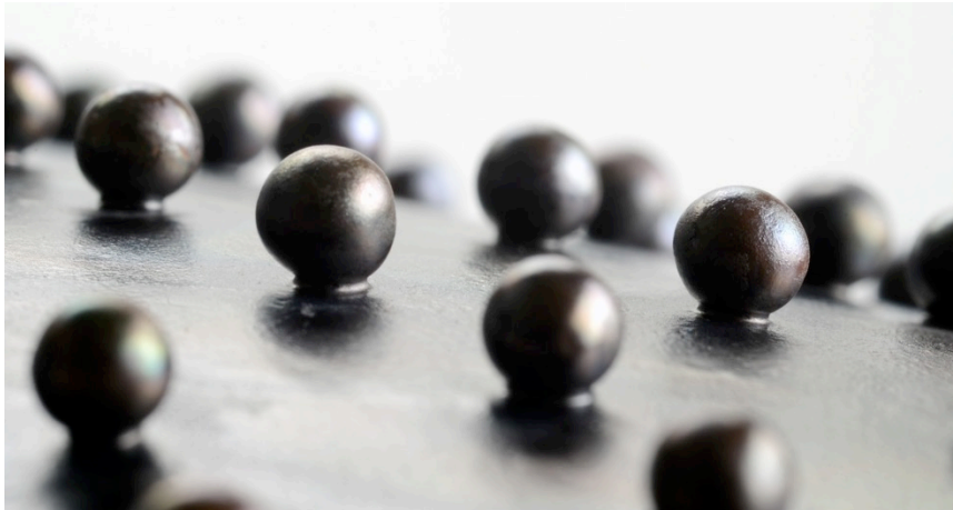
Figure 1: The formation of a neck between the granule and a substrate. 1 The granules are 2 mm in diameter.
