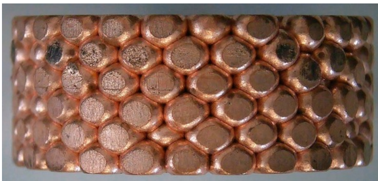
Figure 18: Hot pressed piece made from 3 mm spheres.
