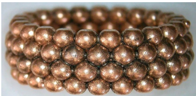
Figure 22: Ring made by liquid phase sintered 3 mm spheres deformed approximately 20% with a platen press.
