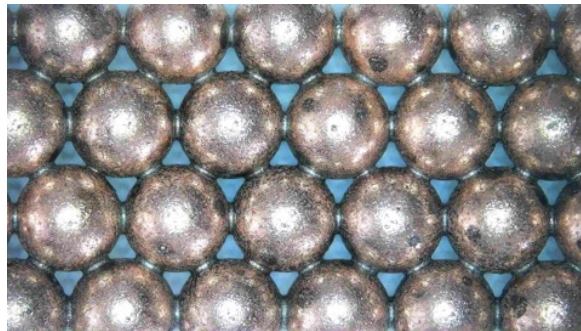
Figure 20: Assembly of 3 mm spheres liquid phase sintered.
