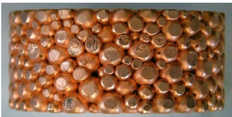
Figure 19: Hot pressed piece made from mixed spheres.
