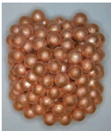
Figure 6: Cylinder made from 3 mm spheres loose sintered in a graphite mold.
