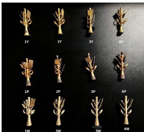
Figure 2: Castings appearance after investment removal
