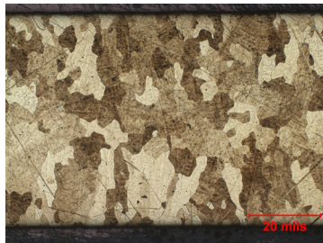
Figure 13: Photomicrograph showing the grain structure of 2W (iridium), HCl-chromic acid etch, 50X original magnification
