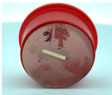
Figure 3: Mounted sample of 1Y for microstructure analysis
