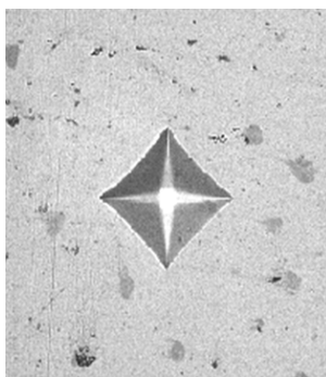
Figure 16: Impression of an indentation on the 18KY gold surface
