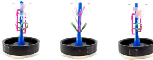
Figure 1: Wax model of casting tree
