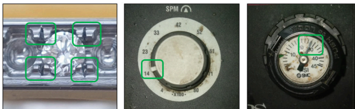
Figure 40: Graver smith correct parameters (SPM & Pressure)
