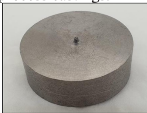
Casting Ingot – \varnothing 28mm
