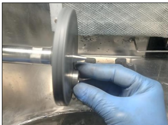
Figure 15: Manual Finishing by felt pad
