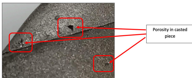
Figure 51: Porosity of Ti Casting
