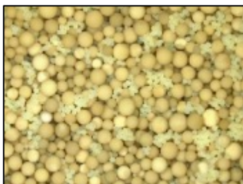
Figure 54: Electrolyte- DLYTE MIX MSA PLUS – S Ti 01
