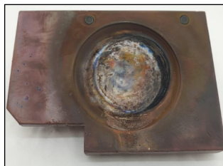
Copper Crucible - \varnothing 42mm
