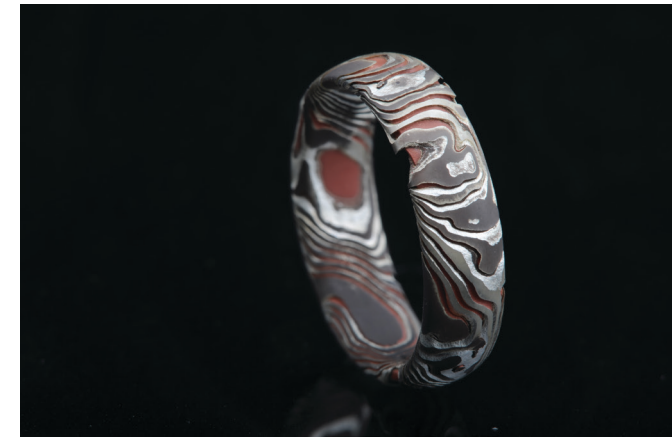
Figure 5: Day 10, ring is severely etched
