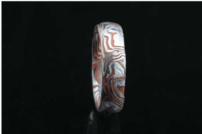
Figure 4: Day 7, ring is deeply etched
