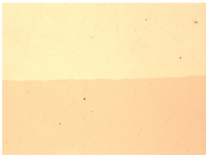
Figure 20: 12-hour billet, unetched, looks like no diffusion across faces, magnification x 200
