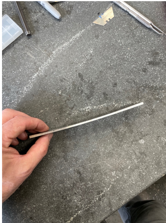
Figure 10: Machined Part That Was Not Annealed (note curve and thicker ends)
