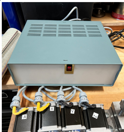
Figure 20: a 4 axis Control box and 4 stepper motors using off-the-shelf parts
