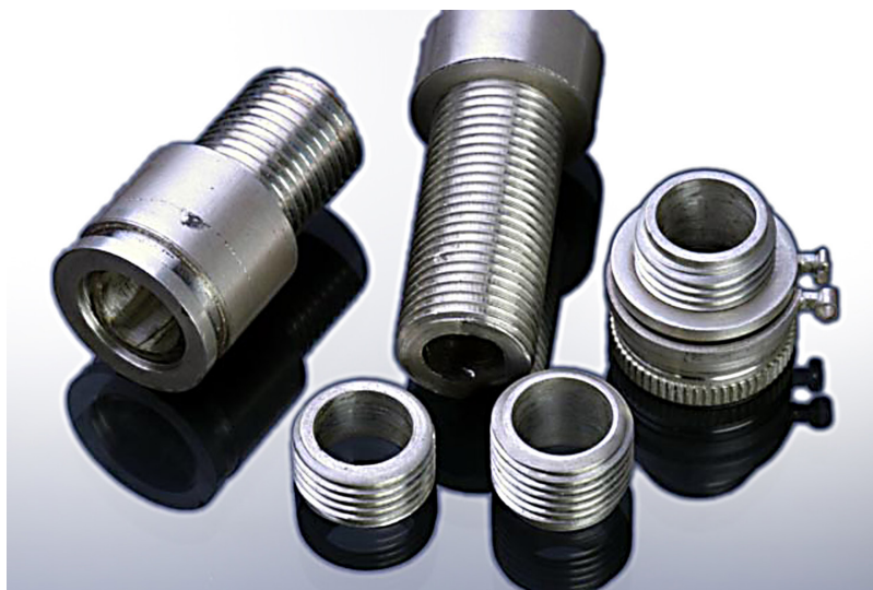
Figure 4: note the threads cut into the sterling silver sand castings
