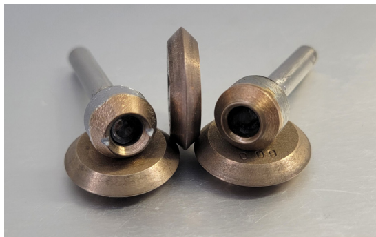
Figure 32: Sintered diamond cutting tools for gemstone carving made at Chris Ploof Designs
