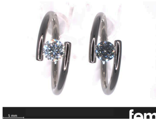
Figure 7: Finished jewelry produced by amorphous investment casting of alloy B with a spring-loaded zirconia stone.
