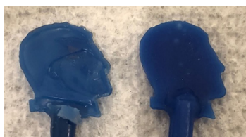
Figure 60: Hybrid solid and hollow wax injection
