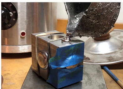
Figure 13: Prepared pre-poured sides sections to pour channel sections D and E
