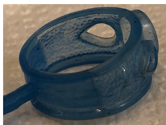
Figures 67 and 68: stipple finish on the inside of ring (left), following nugget valleys inside ring, Combine International, Troy Michigan
