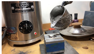
Figure 10: Pouring the first side section of the ring mold
