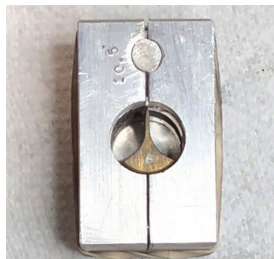
Figure 20: Brass spit plug slide centered correctly inside mold before pouring the core
