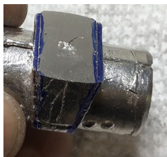
Figure 23: Prepared split plug core for removing side walls to establish wall thickness
