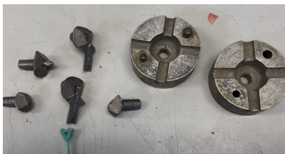
Figure 69: Round mold with five inserts for injecting a 4 prong stone setting, from 1930s era, Jewel Craft, Inc. Erlanger, Kentucky
