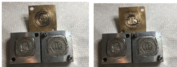
Figures 49 and 50: Finished coin mold with Eddie Bell portrait side (left) and TJS side of model (right)
