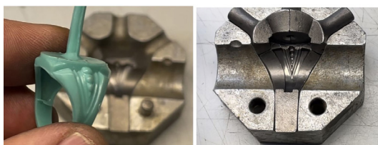
Figure 70: Six sided mold with five parts for wax injection from early to mid 1900s, Jewel Craft, Inc. Erlanger, Kentucky
