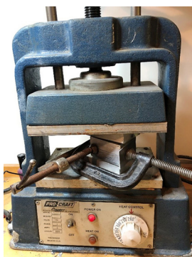
Figure 16: Ring mold being pressed in a heated vulcanizer
