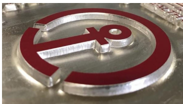
Figure 42: Magnesium photo-etched plate from Owosso Graphics, Inc.
