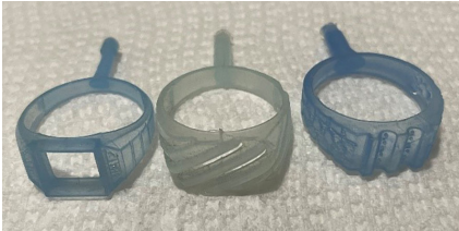
Figures 65 and 66: Three thin-walled ladies rings (left), three thin-walled gents rings (right), Combine International, Troy Michigan
