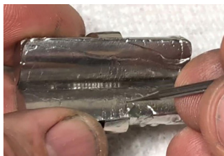
Figure 31: Drilling into underside of core to help break it into two halves
