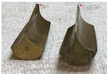
Figure 21: Brass split plug slide, on the right side, filed to a point.
