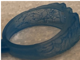
Figures 67 and 68: stipple finish on the inside of ring (left), following nugget valleys inside ring, Combine International, Troy Michigan
