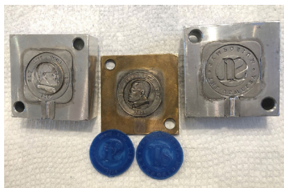
Figure 51: Finished coin model showing wax injections of both sides of the coin
