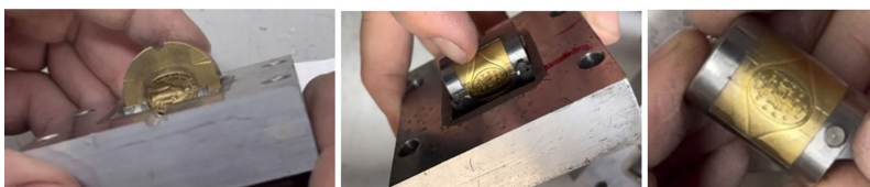
Figure 72: Pressed metal mold with CNC milled plug and top insert for a signet ring that has detail engraved on the inside and outside of the ring. Jewel Craft, Inc. Erlanger, Kentucky
