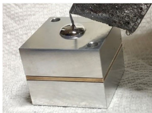
Figure 47: Pouring 1st half of coin mold
