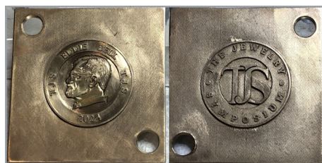
Figure 45: Finished bronze model for TJS coin, this model is 2-sided
