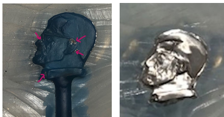
Figure 58 and 59: Wax showing thin spots (left) and finished hybrid core (right)
