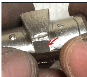
Figure 22: Ring shank core ends filed at an angle to meet the brass slide
