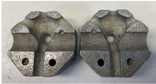
Figure 2: 6-sided aluminum mold frame
