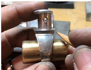
Figure 8: established correct angle on top poured section of the mold
