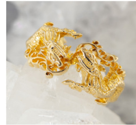
Figure 4: A finished model that was made in ZBrush, and 3D printed and cast in gold
