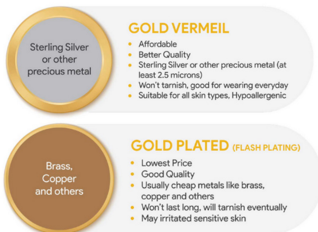
Figure 6: Differences between vermeil and flash gold plating
