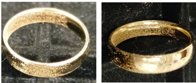
Figure 4: Example of a poorly prepared surface area after gold plating deposit causing delamination
