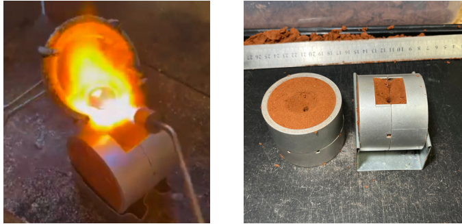
Figure 16: Pouring Molten Metal (left), Top-Pour and Side-Pour Flasks (right)
