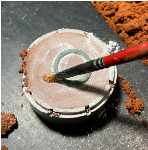
Figure 12: Wax Model is Pressed Halfway into the Sand and Baby Powder is Brushed Over the Top
