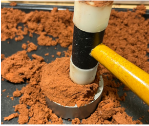
Figure 11: Sand packed into the Male Side of the Flask
