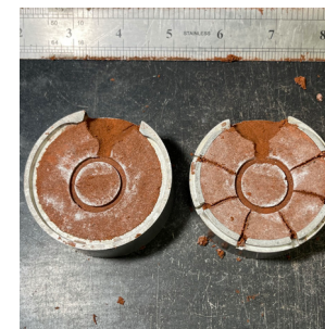
Figure 15: Add the Sprue and Vents
