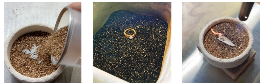
Figure 3: Deep Vermiculite Burial (left), Coconut Carbon (middle), Torch-Firing on Vermiculite (right)
