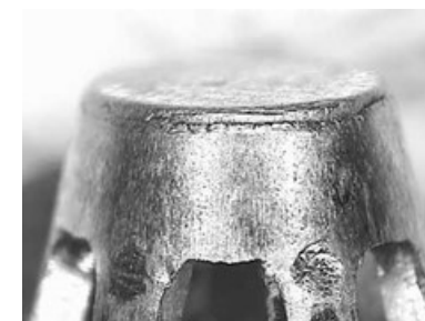
Figure 16: Cracking due to overworking during stamping (Klotz & Grice 5 )
