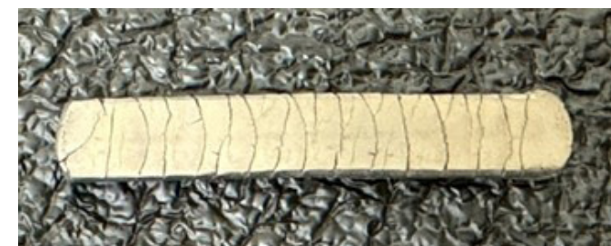
Figure 4: Cracking of a 500-palladium alloy ingot on working due to silicon embrittlement (Binnion 12 )
