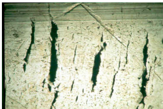
Figure 7: Cracking on the surface of a ring made from continuously cast 14K gold \times 20 mag. (Ott 3 )
