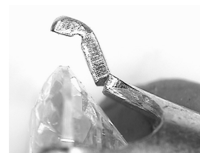
Figure 20: Stress corrosion cracking of a prong in a 14K gold (Grice 18 )
